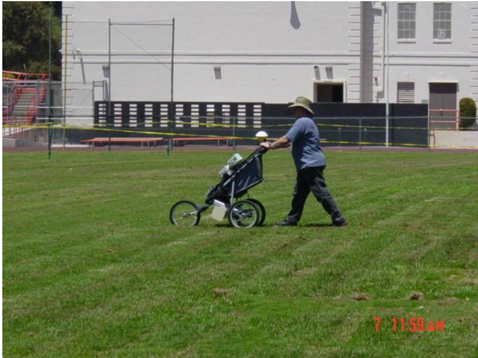
Figure 2: Radiation Data Logging System on Track Field
