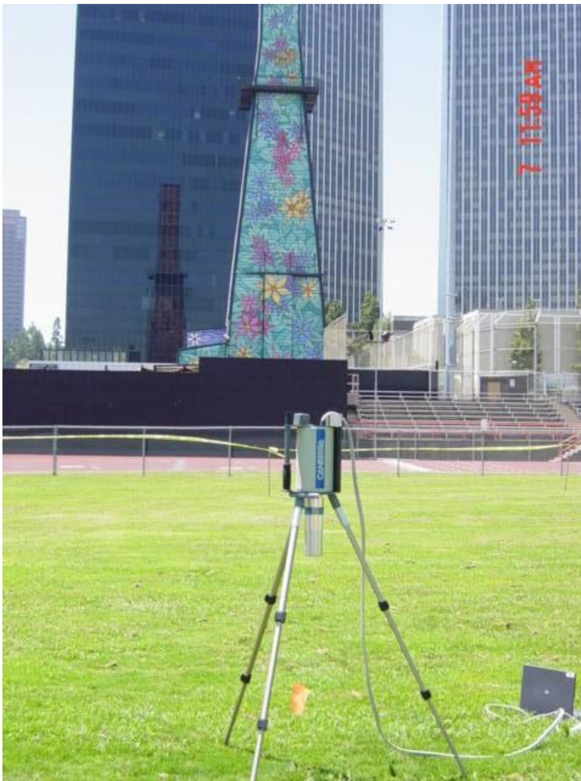
Figure 6: High Purity Germanium Detector In-Situ Measurement on Track Field
